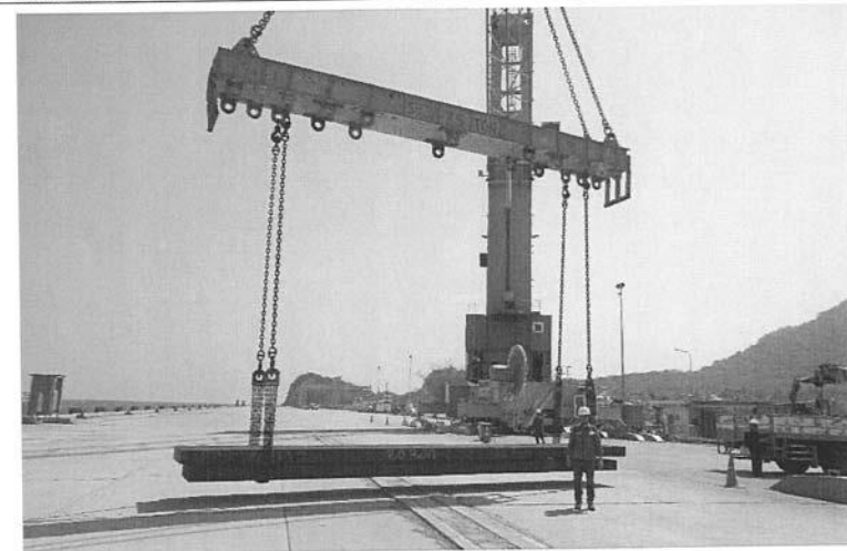
Load testing with Inspection engineer
