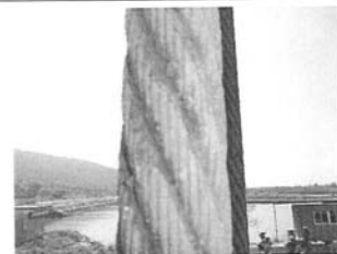
The wire rope shows slight wear, but is otherwise in a normal condition
