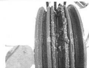
Wire rope : Normal condition
