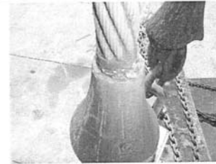
The wire rope shows slight wear, but is otherwise in a normal condition
